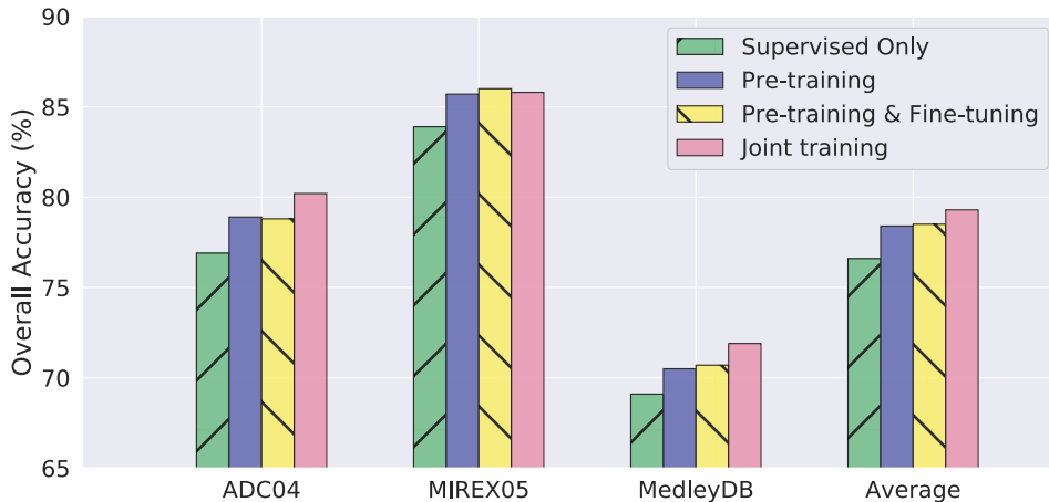
Figure 6.3: Comparison with pre-training, fine-tuning, and joint training methods on three test sets.
